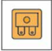
Symbol "Fuse box with fuse for high-voltage deactivation" in the rescue data sheet
