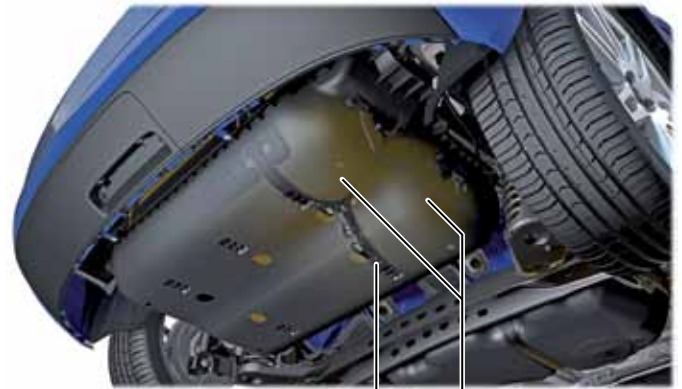
Tensioning belt with protective layer Natural gas tanks
